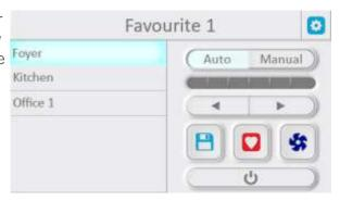
If Zones are locked during the original setup process, the locked Zones will be locked across all Favourites. However it is possible to make alternate Favourite configurations from the Base Screen prior to locking the Zones, then go back into the Advanced Zone Set Up and lock Zones. This allows for more than one 'locked' Favourite setting. Any default Favourites will have all Zones locked to the default position.
