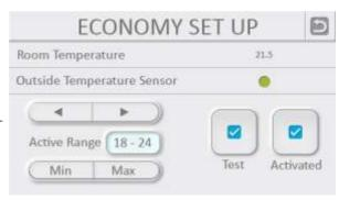
NOTE: The displayed Room Temperature is an average of all the active room Sensors, (also displayed on the Diagnostics screen).
