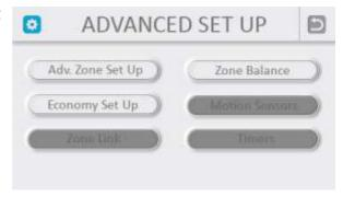
2. Advanced Zone Set Up Zones can be locked so that the end user cannot change zone settings from the Base Screen.
