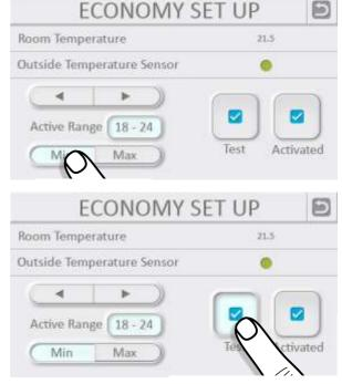
Ensure 'Test' is cancelled and the mode is 'Activated' when the set up is completed.
